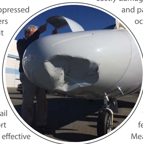
A deer strike caused $100,000 in damage to this aircraft.
